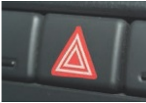
hazard warning light switch
