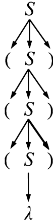
Fig. 1 Derivation tree for the string ((())) , generated by G_{(n)^n} . The axiom is placed on the top, as the root of the tree. The axiom is always the root of all derivation trees derived by a grammar. Notice that the derivation tree hides the order in which rules are applied. Each possible choice is a different derivation. In this case there is only one possibility: the derivation represented in short as S \Rightarrow *((()) and in detail as S \Rightarrow (S) \Rightarrow ((S)) \Rightarrow (((S))) \Rightarrow ((()))
